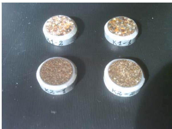
Fig. 3. Specimens of heavy minerals' fractions bonded with polymer resin and polished ("briquettes").
