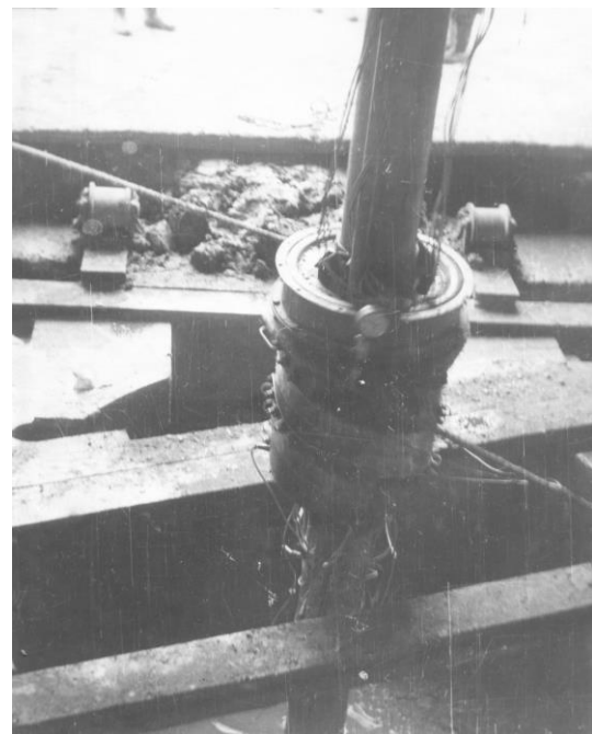
Fig. 3. Collector of sliding contacts (CSC), placed on the upper drill pipe of 10¾ inches with airlift pipes.
