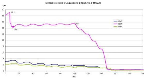
Fig. 4: Current in metal connection at point 1
