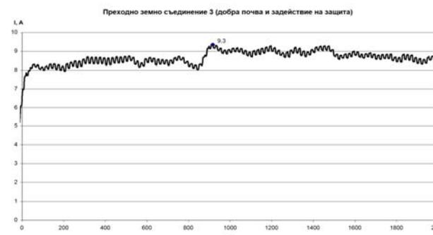
Fig. 3. Current in a transient ground connection at point 2
