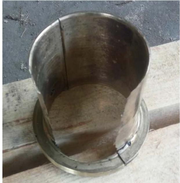
Fig. 4. Wear of plain bearing bush AM8Д
