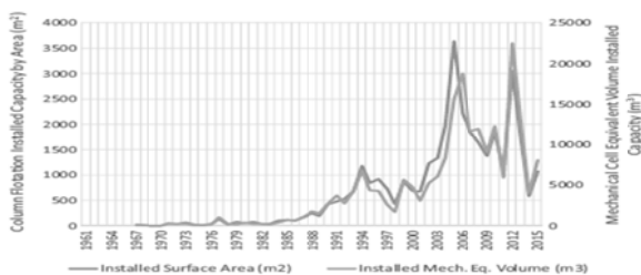
Fig. 4. Column and mechanical flotation machines installed capacity
