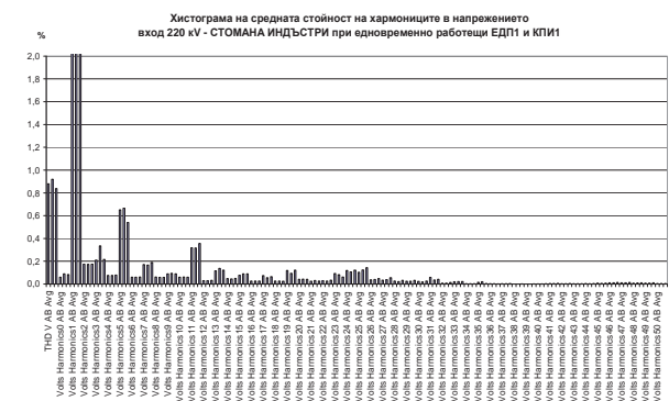
Fig. 6. Bar chart of the mean value of the voltage harmonics - 220 kV input – STOMANA INDUSTRY, EAF1 and LF1 operating in parallel
