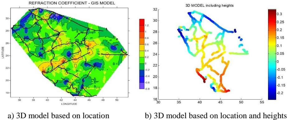
Figure 5.1 GIS models of refraction coefficient
