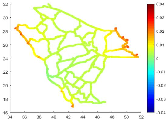
Figure 5.9. Differences of KSA-VRF14 (fixed Jeddah TG) standard deviations (formal errors) with regard to standard deviations of combined solution(all TG fixed) heights from TG&SA analysis. Units: [m]
