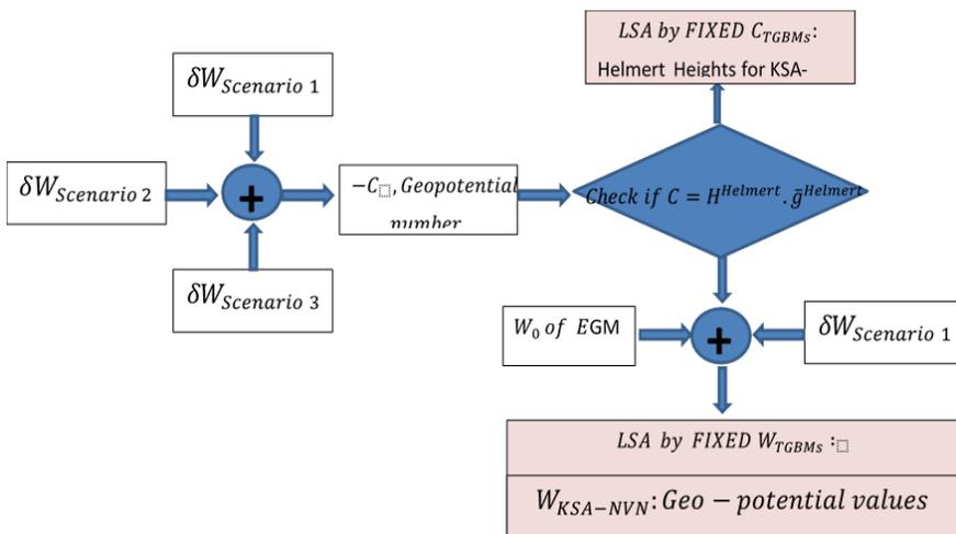
Figure 5.11. Block diagram for combining scenarios 1-3 for computing geopotential values and orthometric heights of KSA-NVN BMs
