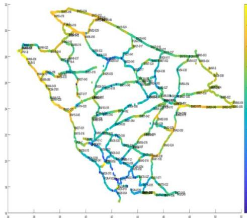
Figure 5.7. GPS/GNSS/Levelling Geoid heights per ~3500 BMs used for computation of  $\delta N [m]$  and  $\delta W [m^2/s^2]$ : Colure range: -1:1 meters
