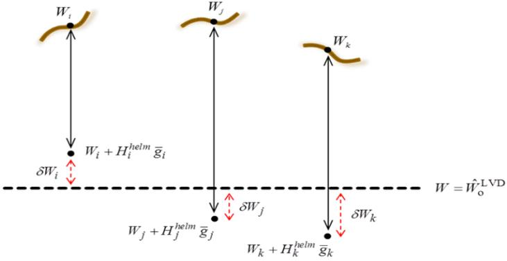
Figure 3.22. Zero-height geopotential value determination from a network of stations.
