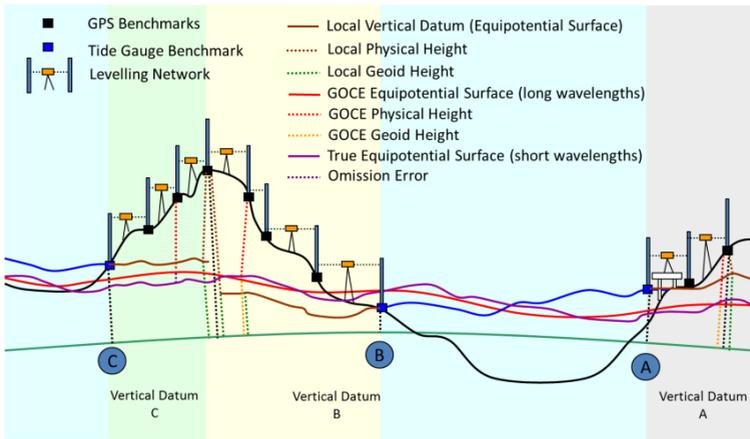
Figure 3.23. LVDs and GOCE-based geoid aid to LVD unification (Gruber et al. 2014).
