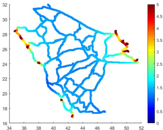
Figure 5.10. Ratio of formal errors from KSA-VRF14 (fixed Jeddah TG) heights over the formal errors of combined solution (all TG fixed) from TG&SA analysis. Units: [no units, just ratio]
