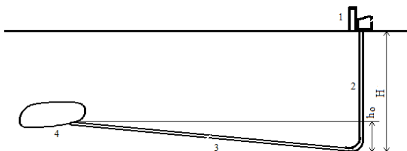
Fig. 4. Scheme of vibration-gravity pipeline transport of hardening mixtures: 1 – filling complex; 2 – well; 3 – cross-cut; 4 – man-made voids; H – depth of the filling hole to the earth’s surface, m; h_0 – height of rise of hardening mixtures to man-made voids, m
