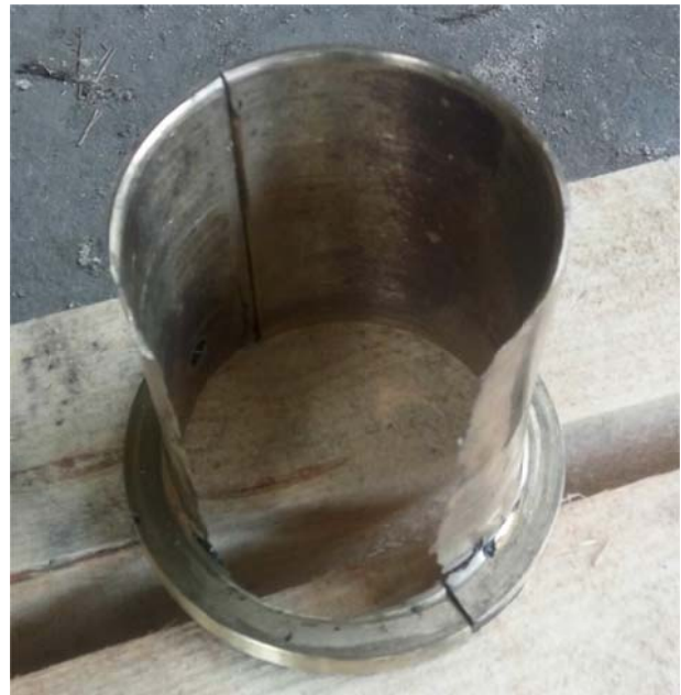
Fig. 4. Wear of plain bearing bush AM8Д
