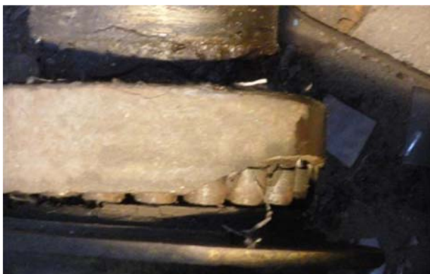
Fig. 3. Destruction wheelset roll bearing K10M
