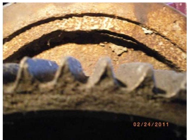
Fig. 5. Gear wear AM8Д
