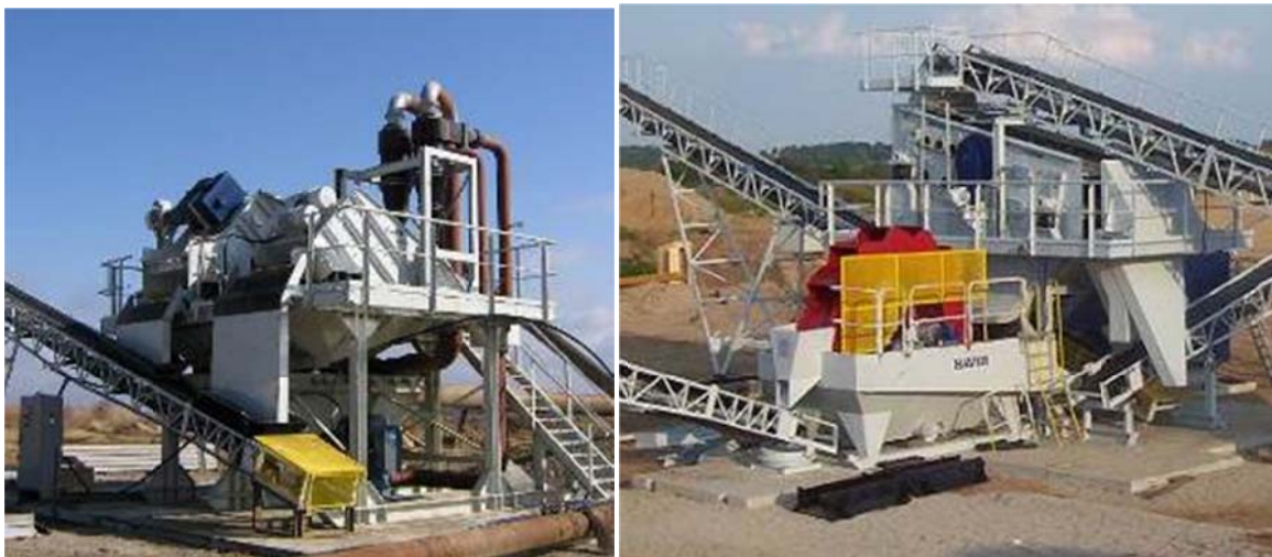
Fig. 11. Sand Recovery System: left Hydro Cyclons in combination with Dewatering Screens, right Bucket Wheel
