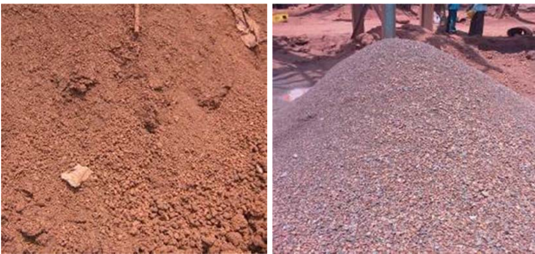
Fig. 9. Iron Ore Fines 0 – 30 mm, left before washing, right after washing
