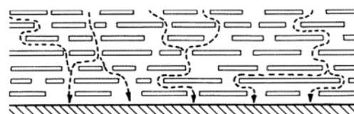
Figure 3. Barrier effect created by MIO particles
