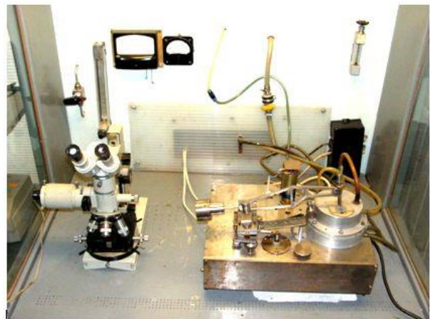
Fig. 4. An experimental sample for the thermochemical method installation: processing diamond (modification PTC "URALALMAZINVEST")
