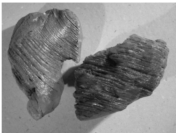
Figure 12. Superficial forms of dissolving along the planes of translation with dynamogenic twins
