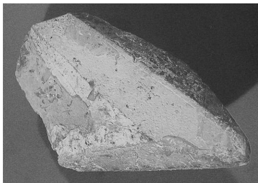
Figure 7. A calcite crystal with a scalenohedron and a hexagonal prism.
