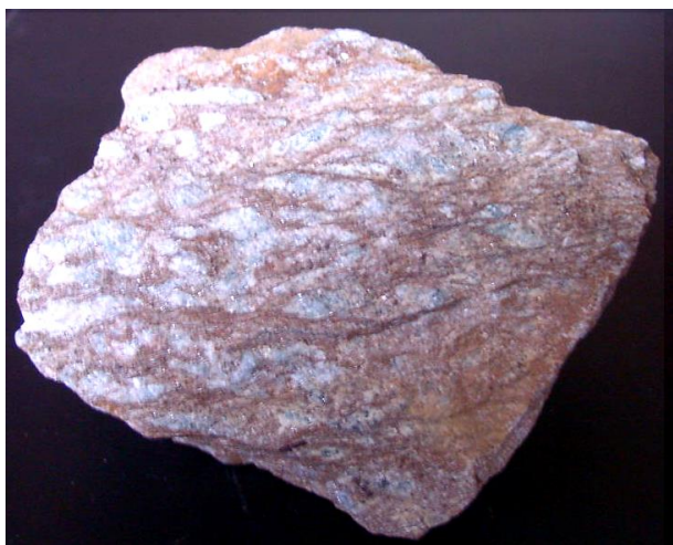
Figure 2. The measured surface of kyanite schist (Specimen 1)
