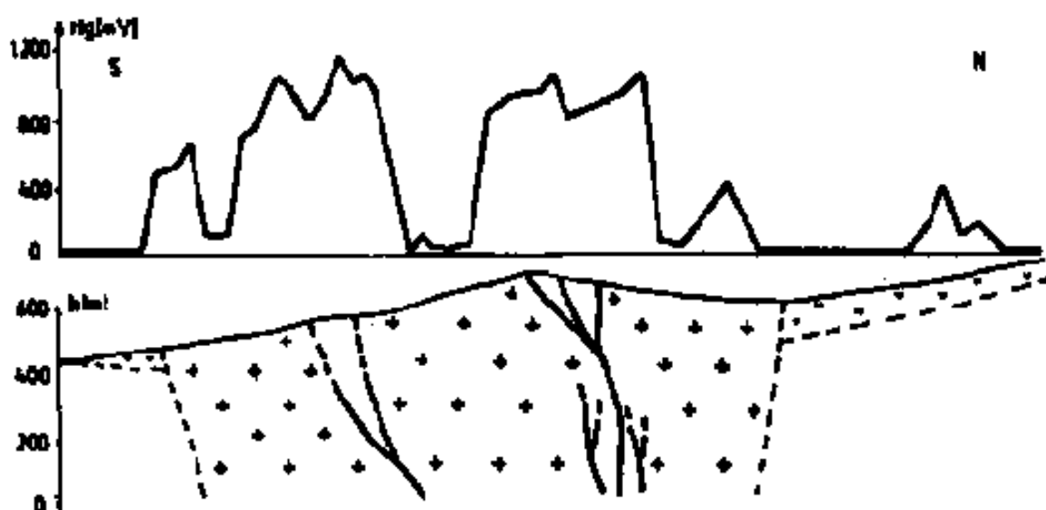
Figure 4. Mercuriometric anomalies across the Baia Sprie Au-Ag ore deposit (Gutai Mts, East Carpathians, Romania)
