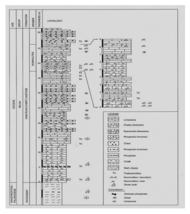
Fig. 2. Columnar lithological section of the Eocene rocks in the study area
