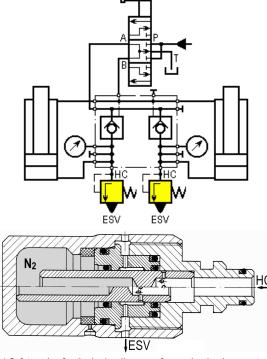
Fig. 4 Safety valve for the hydraulic props for mechanised support
