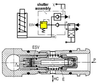
Fig. 3 Individual hydraulic prop shutter for open circuit
