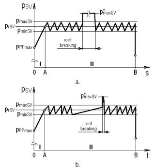
Fig. 5. Operating characteristics of safety valves for hydraulic props: a – opening pressure dynamics  $p_{SV} = f(t)$ ; b – the dependence of the opening pressure on the stroke of the piston of the prop  $p_{SV} = \phi(s)$ .
