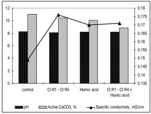
Fig. 4. Application of microorganisms and humic acids on pH, active  $CaCO_3$  and specific conductivity
