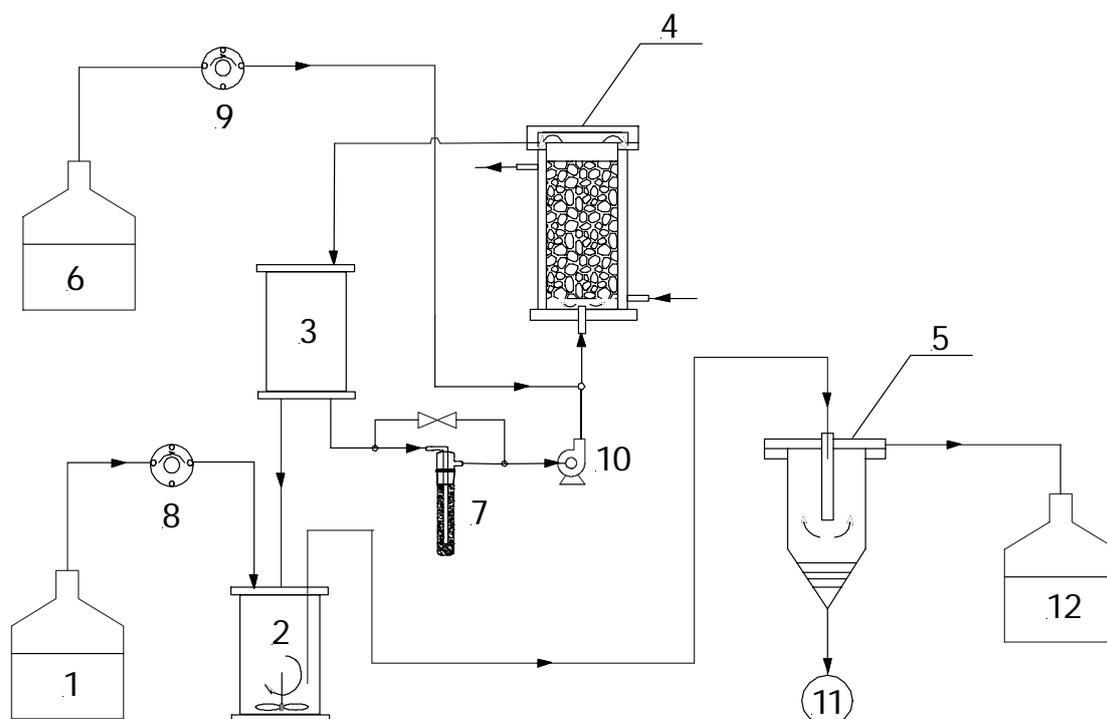
Fig.1. Schematic diagram of the laboratory installation for active treatment of wastewaters polluted with heavy metals. 1 – Heavy metals solution tank, 2 – chemical reactor, 3 - mix tank, 4 - anaerobic fixed-bed biofilm reactor, 5 – settler, 6- nutrient medium tank, 7- sand filter, 8 and 9 – peristaltic (roller) pump, 10 – recirculating pump, 11 – sludge, 12 – collector tank.
