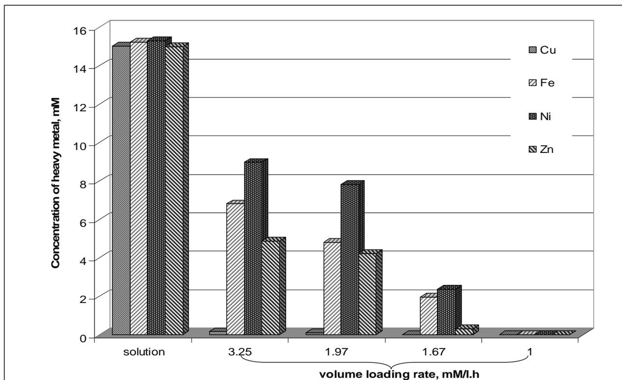
Fig. 3. Removal of Cu, Fe, Ni and Zn ions with initial concentrations 15 mM at different volume loading rates of the chemical reactor
