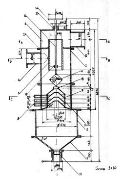
Figure no.3 Additional water flow hydrocyclon - HCCAD 400
