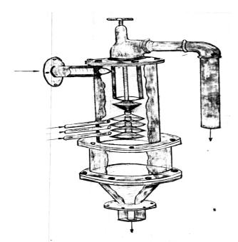
Figure no.1. - Additional water flow hydrocyclon
