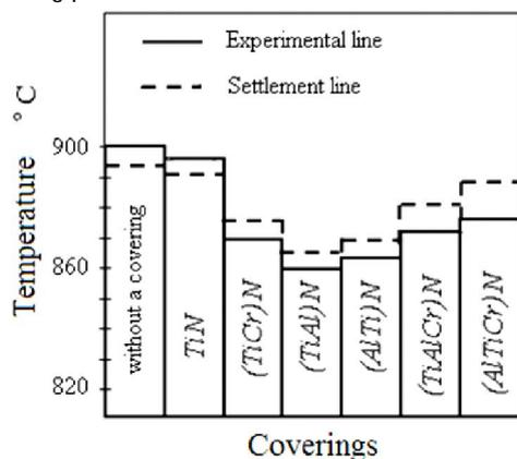
Fig. 2 Influence of a covering on cutting temperature at the turning
