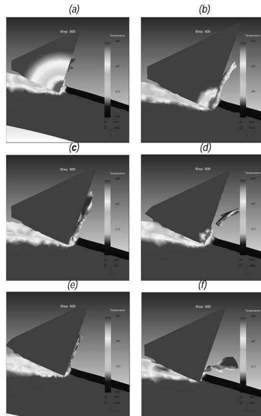
Fig. 1 Calculation of temperature fields at the cutting in the software «DeForm 3D»
