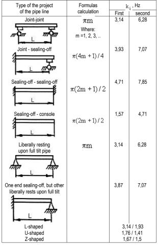
The tension axis effort increases the own frequency, and decreases it with respect to the pressure. This fact is of significant importance for the determination of the first form of the variations. As for pipes of two knuckle bearings, the importance of the first own frequency with reporting of the axis strength N is being determined according to the following formula:
