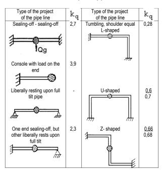
As for pipelines with a great number of sections of equal lengths, the own frequency is being calculated according to the following formula: ,
