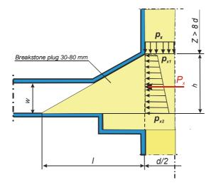
Fig. 1. Computational diagram applied to determine the slope length of the shaft plugs
