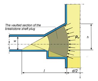
Fig. 2. Hypothetical artificial vault in the shaft plugs
