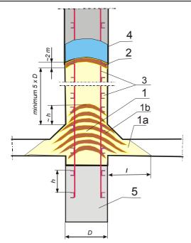
**Fig. 3. Scheme of a shaft plug aggregated with concrete** 1 – hardcore or hardcore free draining plug, 1a –gallery section of the plug, 1b – shaft section of the plug, 2 – stone-concrete layer that protects the plug from the clay material, 3 – structure of the shaft reinforcement, 4 – clay insulation plug, 5 – unsorted rock material
