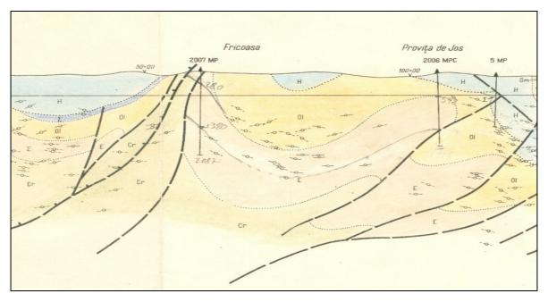
Fig. 3.. Cross-section of the northern border of Diapiric Fold Zone
