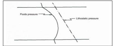
Fig. 2 . Fluids pressure distribution in a thick clay layer after Chapman 1976, with modifications
