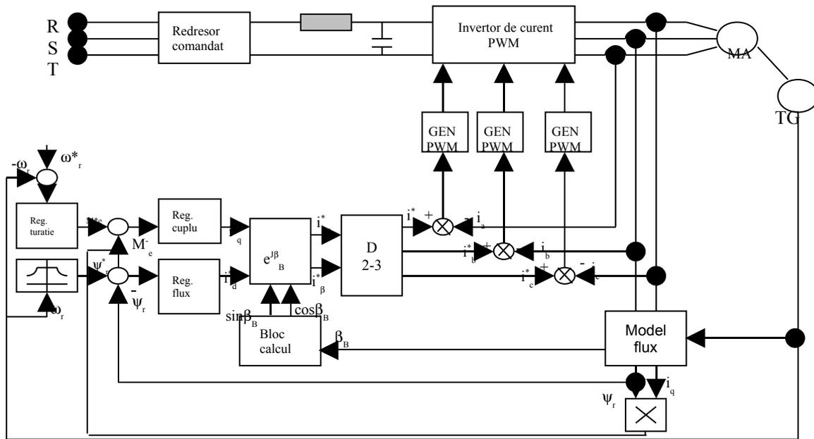
Fig. 4. The block scheme of adjustment with field orientation of the revolution of an asynchronous motor powered by a PWM current inverter
