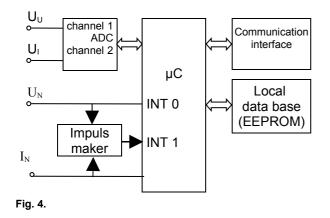
The system with  $\mu$ C controls the acquisition of the current and potential signals, and, also measuring with the help of the two intern timers the duration of the potential signal for the calculation of the frequency and also the duration between the appearance of the potential and current impulses.
