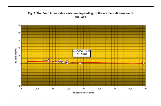
It come out that at the same standard diameter with a ball charge near the standard average value, resulted index is higher than obtained with standard charges, but the variation is insignificantly.
