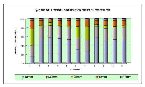
From point of view of weight composition, presented in figure 2, is seen a reduced quantity of small balls comparative with coarse balls, the average classes being representative in experiments 1, 6 and 7. In all other experiments, balls with diameter value of 40mm represent higher than 50% in charge weight.
