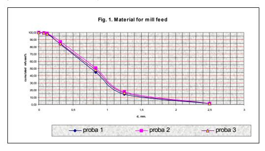
The samples were tested complying with a pre-established program, following all the stages of the test. The program refers to establish the influence of size ball charge, like average size, on Bond index value. In this experiments, the feed sized, the ball charge and the mill revolution were unchanged.
