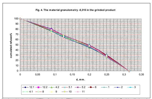
Crossing point with straight of 20% ordinate (passing 80%) determines  $\,$  Xp,  $\,$  material  $\,$  size  $\,$  -0.315mm  $\,$  resulted  $\,$  from
