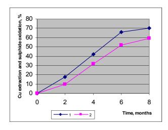
Fig. 1. Leaching of copper (1) and degree of sulphide oxidation (2) during the treatment by means of chemolithotrophic bacteria
