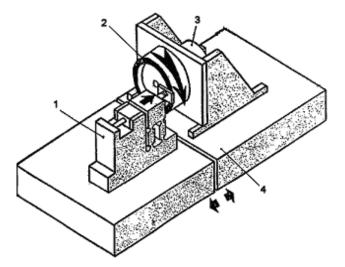
Fig. 2. Diagram of PEGASUS. 1 -work fixture; 2 - abrasive disk; 3 - spindle; 4 - dovetail slide.
