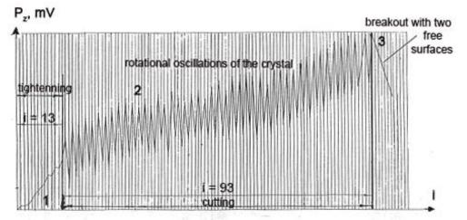
Fig. 1. Experimental oscillogram of alteration of the cutting force normal component. 1 - section of the stressing (tightening) accumulation; 2 - section of the transient process; 3 - section of stationary regime; P<sub>z</sub> - normal component of the cutting force; i - number of the working paths.
