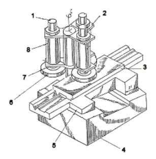
Fig. 3 Machine for dimensional microgrinding with three cutting tools. 1 – motor; 2 – cutting tool fixture; 3 – stop; 4 – frame; 5 – slide; 6- cutting tool; 7 - cutting tool fixture; 8 – drive of rotation.
