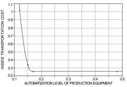
Fig. 5: Diagram of the relation between the automation level and the inside transportation costs.
