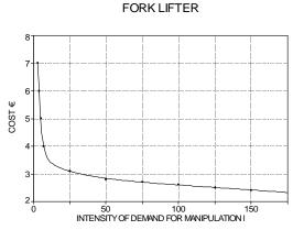
Fig. 3: Exploitation cost of a fork lifter as a function of intensity of demand for manipulation
