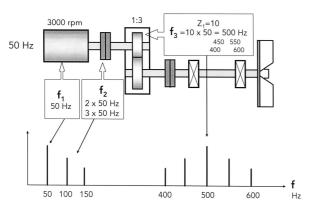
fig.1. Spectrum lines, first shaft
