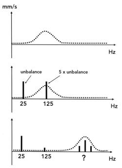
fig.4. Amplitude of spectrum line
