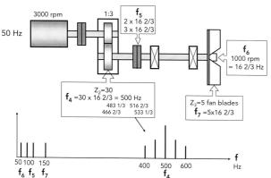
fig.2. Spectrum lines, second shaft
