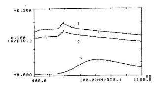
Figure 1. Electronic spectra of borate ruby glasses. Copper was introduced as a CuO and was used an organic reducer. Melting duration: 1 – 15 min., 2 – 30 min., 3 – 60 min.
