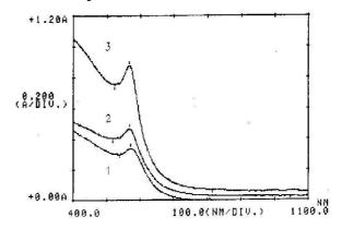
Figure 2. Electronic spectra of borate ruby glasses with copper from a Cu-Sn alloy. The heath treatement duration was: 1 – 120 min.. 2 – 210 min.. 3 – 240 min.
