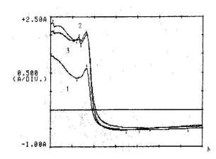
Figure 3. The electronic spectra of the industrial type ruby glasses with alloy, maintained at the melting temperature: 1
