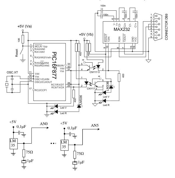
Fig. 2. The electronic signal acquisition diagram
