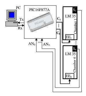
Fig. 1. The block diagram used for temperature monitoring
