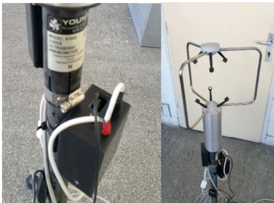
Fig.3. Anemometer with the attached controller box
