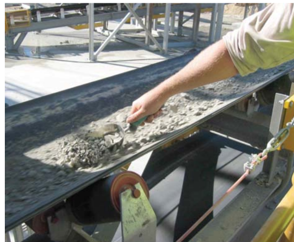
Fig. 1. Sampling from the top of conveyor belt (Holmes, 2010)
