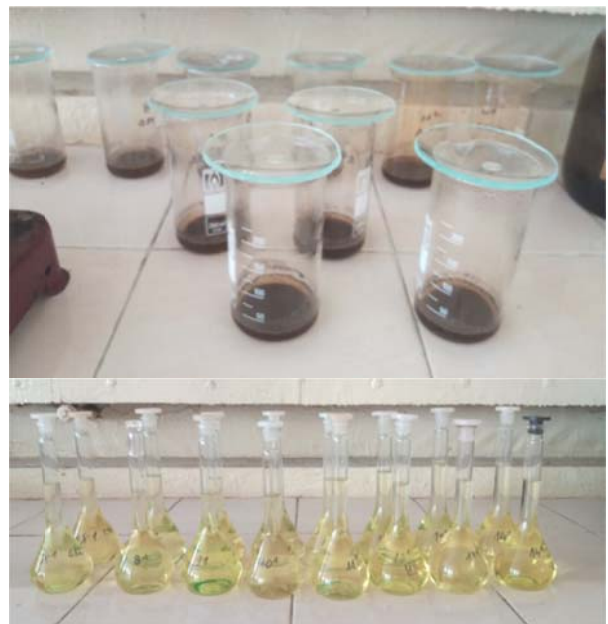
Fig. 9. Preparation of the samples by the method of acid dissolution
