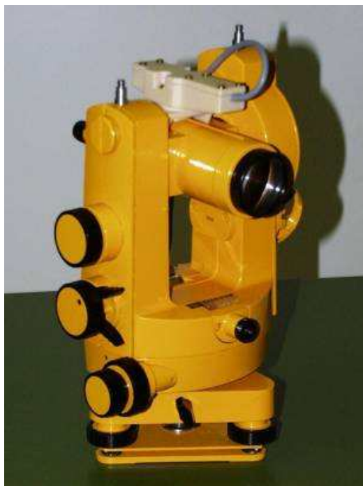
Fig. 1. DI Flux magnetometer - theodolite with Fluxgate sensor on the top
