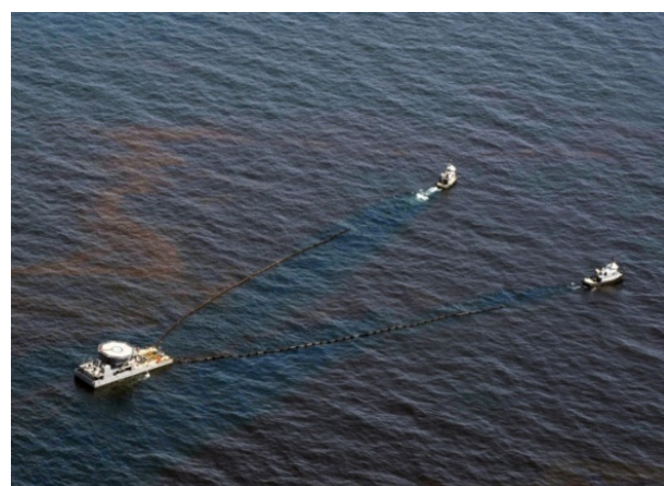
Fig. 16. Offshore oil boom deployed in a "V" configuration (IOGP Report 522, 2015)
