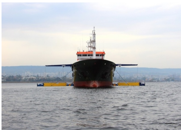
Fig. 19. Oil collection system via sweeping arms
