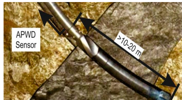
Fig. 2. APWD Sensor position in BHA
