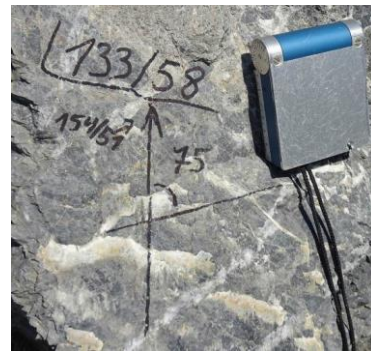
Fig. 8 Example of marking the fault kinematic axes on a fault surface from Tasladja Bair quarry, using the Aki-Richards format, described in the manual of the FaultKin software (Marrett, Allmendinger, 1990) for rakes of striae on planes
