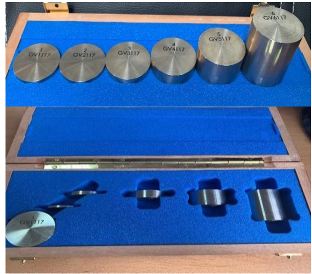
Fig. 4. Reference washers for the Vinci 3.28 helium porosimeter
