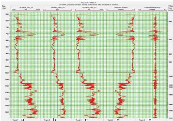
Fig. 6. P-1 Galata well– curves created by the correlated P-wave for the purposes of AVO developed methodologies a/ basic curve P-wave\_corr; b/ density curve from Gardner's – transformation of basic curve; c/ curve of velocities of S-wave from Krief's – transformation of basic curve; d/ curve of Poisson's ratio coefficient; e/ Distribution of reflection coefficients calculated of basic curve
