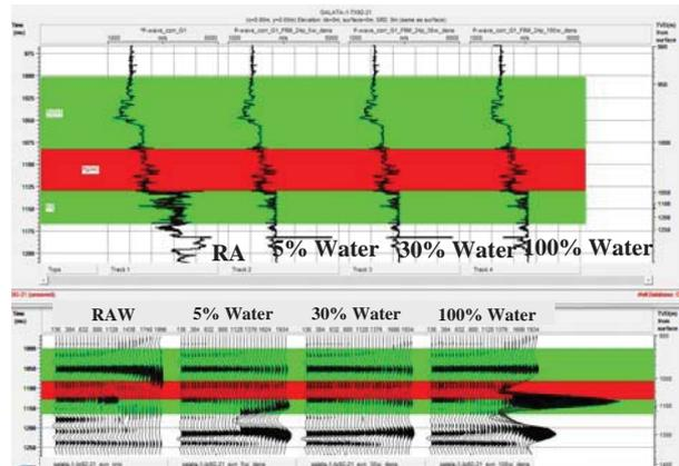
Fig. 7. AVO-modeling at water saturation 5, 30, 100%, constant density 2.22g/cm³ for target area and porosity 24% (P-1 Galata well)
