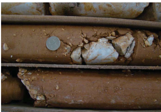
Fig. 2. Core of tectonically reworked limestone nearly completely converted to a clay.
