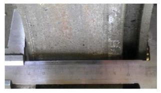
Fig. 2. Wear bearing housing
