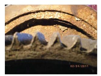
Fig. 5. Gear wear AM8Д
