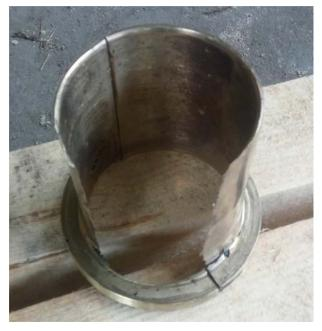
Fig. 4. Wear of plain bearing bush AM8Д
