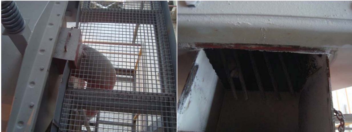
Fig. 9 – Device for lumps removal from vibrating feeder
