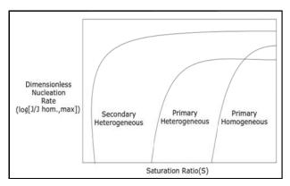
Fig. 4. Nucleation rate vs. saturation ratio S
