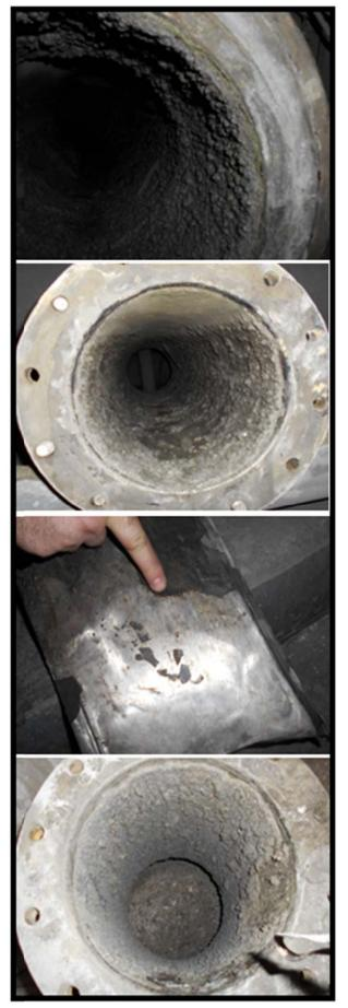
Fig. 3.Gypsum scale formations in the DPM Chelopech flotation plant equipment
