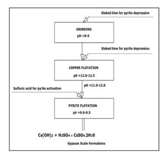
Fig. 2. Addition points of slaked lime and sulfuric acid in DPM Chelopech flotation plant
