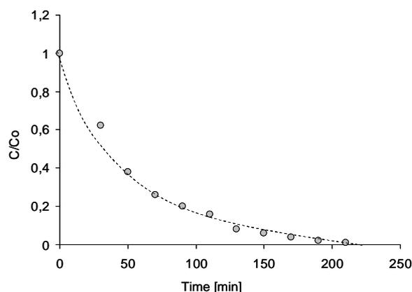
Fig. 1. First-order kinetic trace for the photocatalytic decoloration of Reactive Black 5 at pH = 2.7
