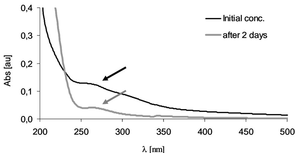
Fig. 2. Absorption spectra of aromatic byproducts of RB5 (pointed with arrows) before and after two days biological treatment by active sludge
