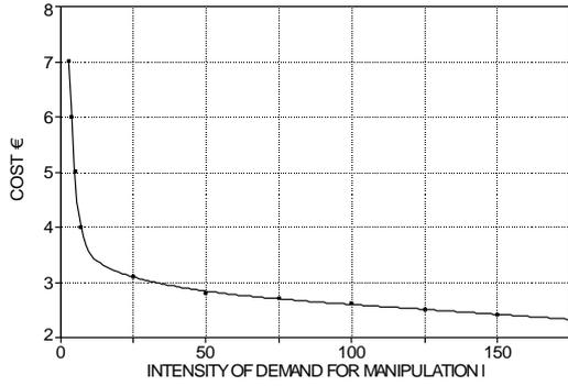
Fig. 3: Exploitation cost of a fork lifter as a function of intensity of demand for manipulation
