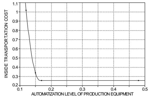
Fig. 5: Diagram of the relation between the automation level and the inside transportation costs.
