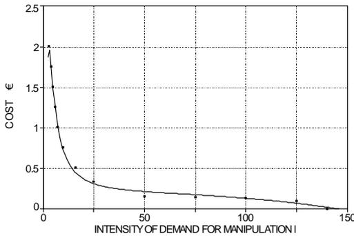
Fig. 4: Exploitation cost of a floor conveyer as a function of intensity of demand for manipulation
