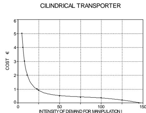
Fig. 2: Exploitation cost of a cylindrical transporter as a function of intensity of demand for manipulation
