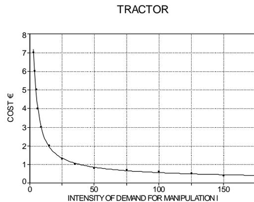
Fig. 1: Exploitation cost of a tractor as a function of intensity of demand for manipulation
