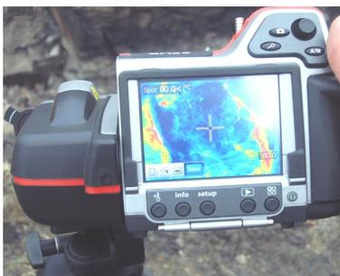
Fig. 2. Thermal vision camera, Flir type
