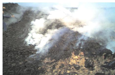
Fig. 3. Pile with self-alight lignite
