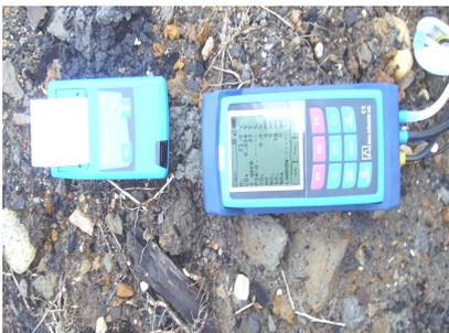
Fig. 1. The measurement kit of the combustion gases analyzer, Multilyzer N.G. 1 – central unit, 2 – sampling probe, 3, 4 – temperature sensors, 5 – tension adaptor, 6 – portable printer with infrared data transmission, 7 – hose for clean air calibration of the apparatus, 8 – transportation bag
