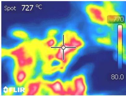
Fig. 4. Maximum temperature registered at the surface of the self-ignite coal pile
