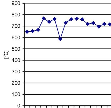
Fig. 6. Measured temperature at the surface of the coal pile
