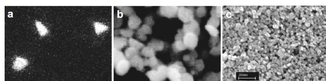
Fig. 2. SEM images of (a) FeO(OH), (b) ZnO and (c) TiO 2 nanoparticles. Scale bar = 200 nm.
