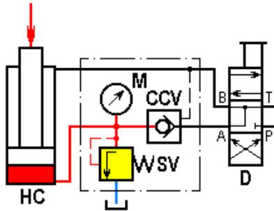
Fig. 1 Face hydraulic prop. Hydraulic basic diagram
