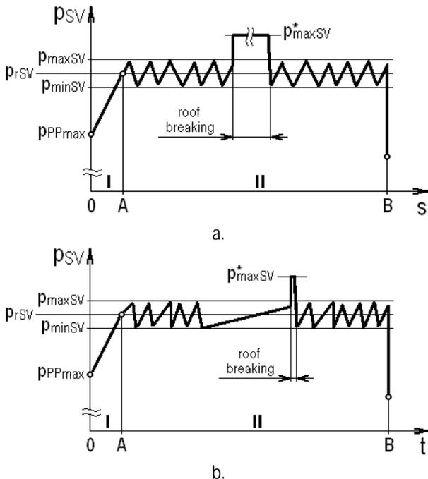
Fig. 5. Operating characteristics of safety valves for hydraulic props: a – opening pressure dynamics  $p_{sv} = f(t)$ ; b – the dependence of the opening pressure on the stroke of the piston of the prop  $p_{sv} = \varphi(s)$ .
