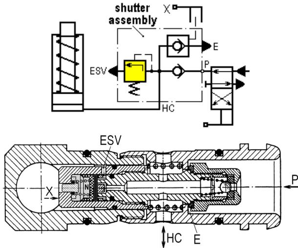
Fig. 3 Individual hydraulic prop shutter for open circuit
