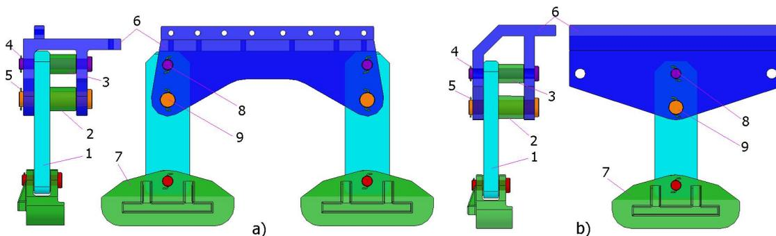
Fig.4. Modifications in the structure of the skid at the front mounted on the reducer and the feed mechanism
