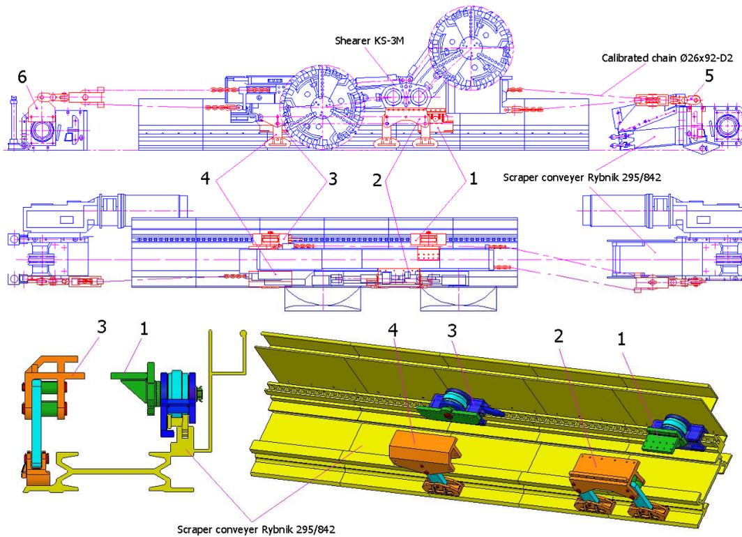
Fig.1. KS-3M feed system for Rybnik 295/842 conveyer
