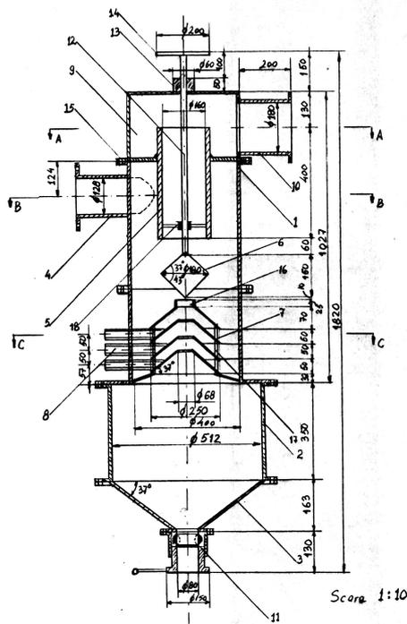
Figure no.3 Additional water flow hydrocyclon – HCCAD 400
