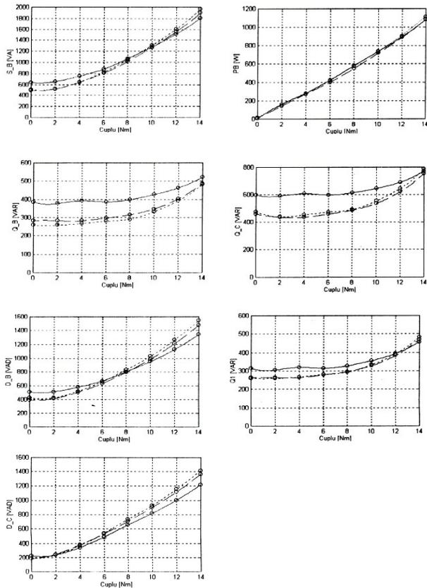
Fig. 8 The dependency of the powers in couple, at  $f=20\text{Hz}$  for: S.A. with M.A. and CSTF cu frequency modulation – continuous line; S.A. with M.A. and CSTF with sinus modulation – interrupted line; S.A. with M.A. and CSTF with the elimination of the harmonics – dotted.
