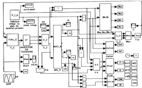
Fig. 3 The Simulink model of S.A. with M.A. and indirect CSTF, tension source with the determination of energetic parameters
