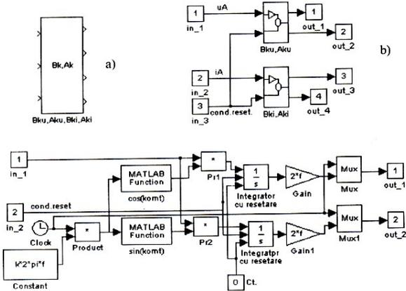
Fig. 1 The Simulink Model for calculating the components amplitude in sinus and cosine of the tension and current harmonics : the mask block –a); it's structure –b); the structure of the blocks “Bku, Aku” and “Bki, Aki” –c)
