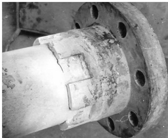
Fig. 9. View of a zone with penetrated macro-crack on the drilling pipe without air tubes, with series 122.
