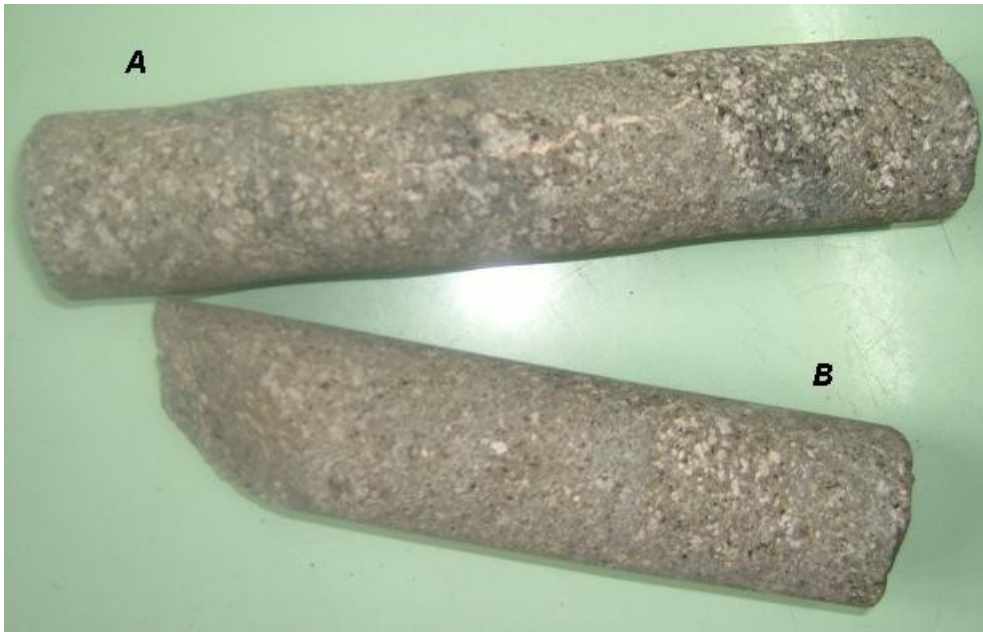
Fig. 6. A - core obtained in drilling without BHSA; B – core obtained in drilling with BHSA
