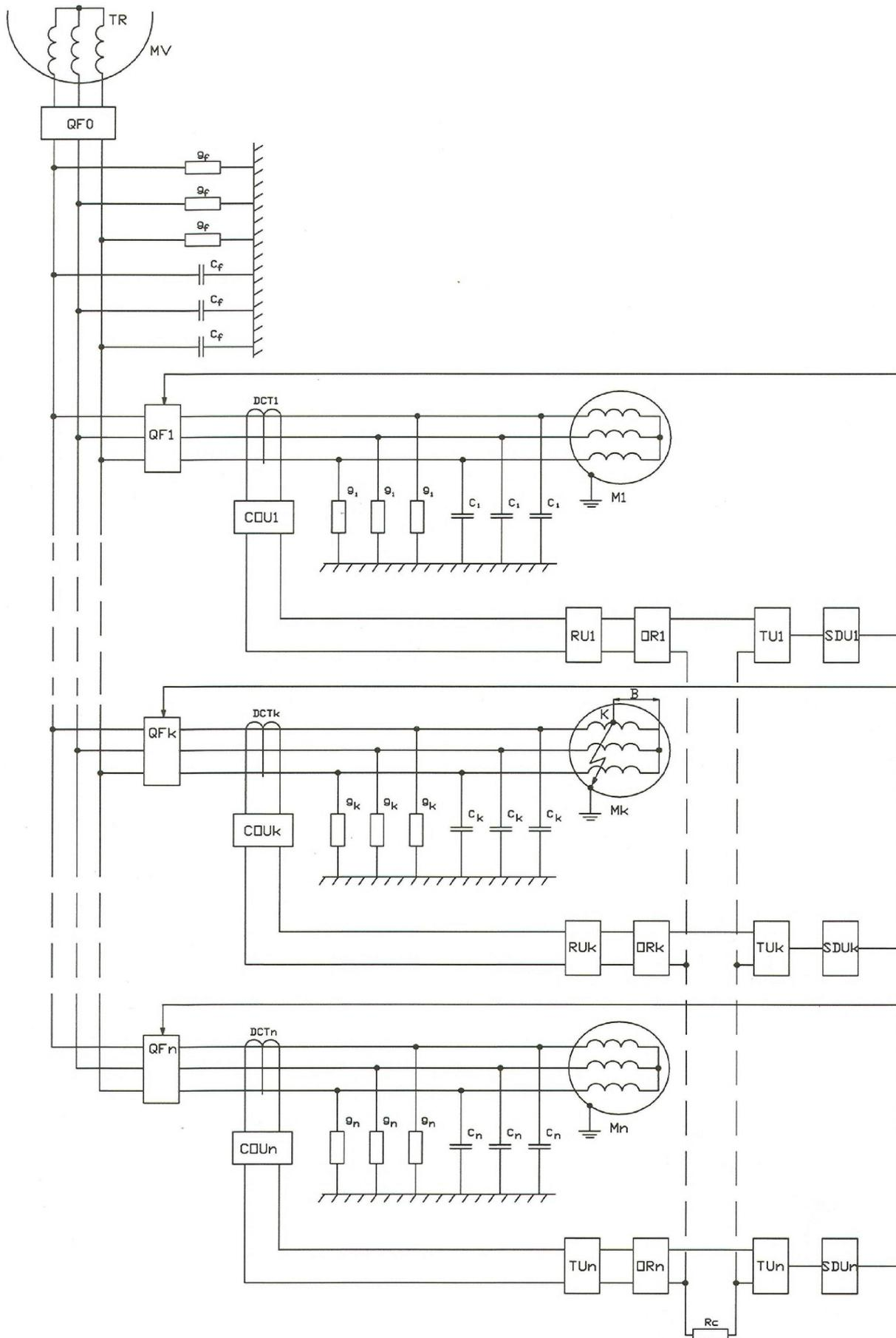
Fig.1. Block diagram of group protection of single phase earth faults for n synchronous motors
